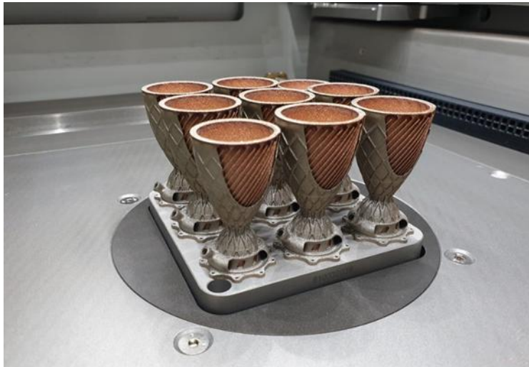
Figure 57: Nickel-copper combustion chamber demonstrator parts on the build platform 99
