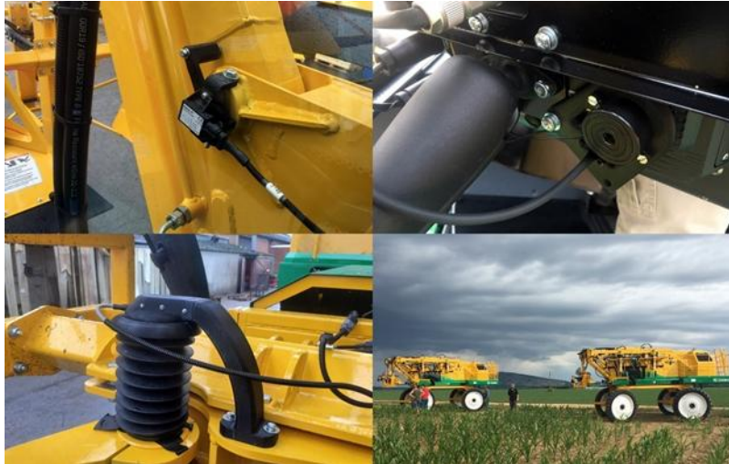
Figure 24: Functional 3D printed components of a heavy-duty agricultural detasseler machine from PMC Harvesters 71
