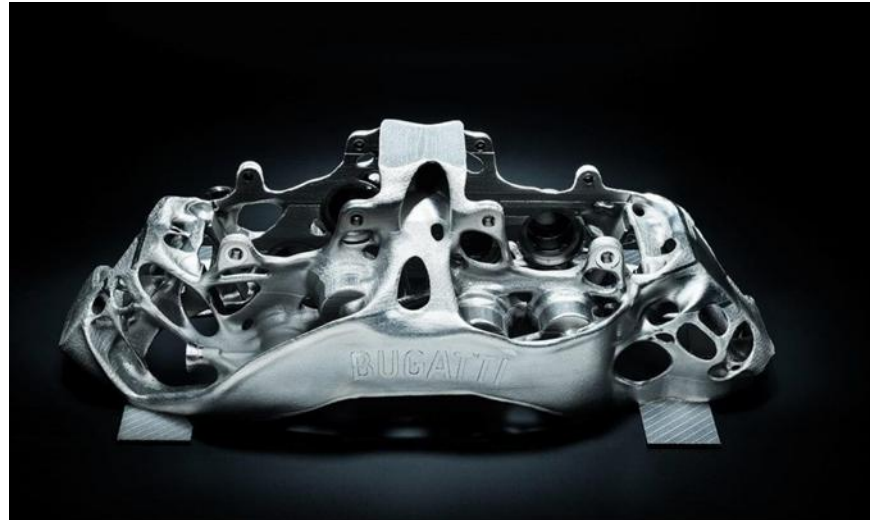
Figure 28: An intricately shaped brake caliper with wall thicknesses between 1 mm and 4 mm for Bugatti Chiron 78
