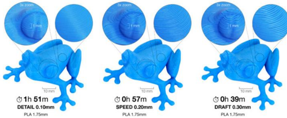
Figure 15: Effect of layer height on quality of 3D-printed part 43
