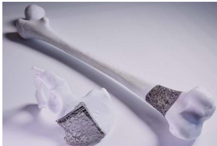
Figure 55: Multiscale structure of bio-implants – osseointegration
