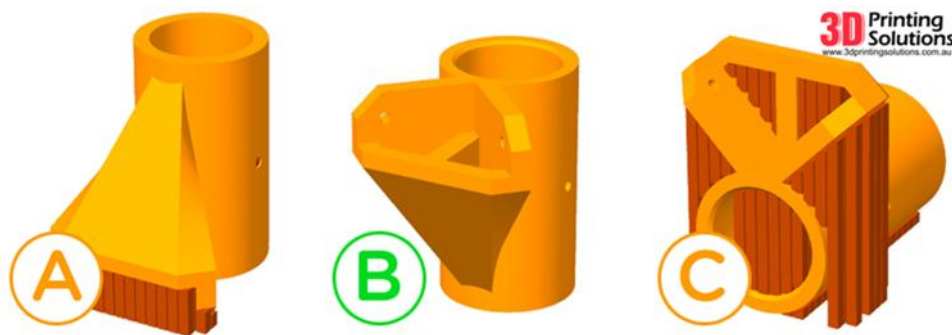
Figure 19: Effect of printing orientation on the amount of supporting material 48
