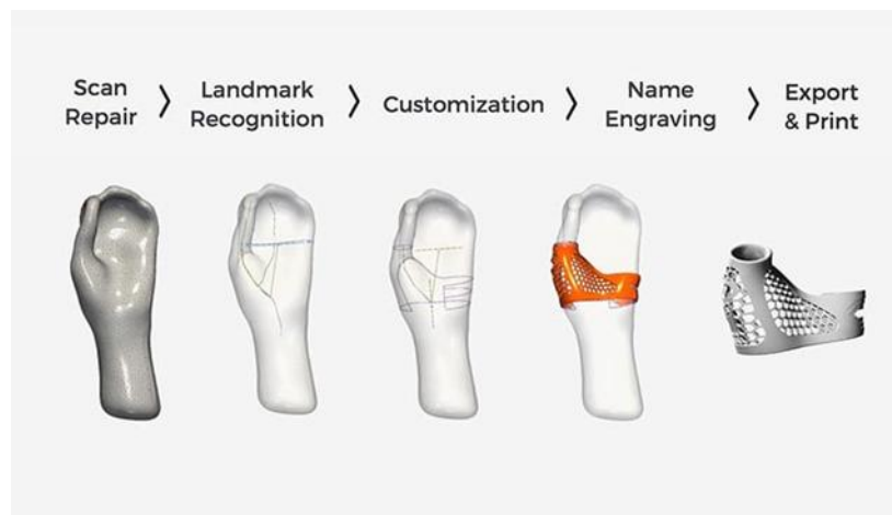
Figure 31: Illustration of typical steps in a 3D printed mass customization workflow of a thumb-prosthetic device by Shapeshift 81
