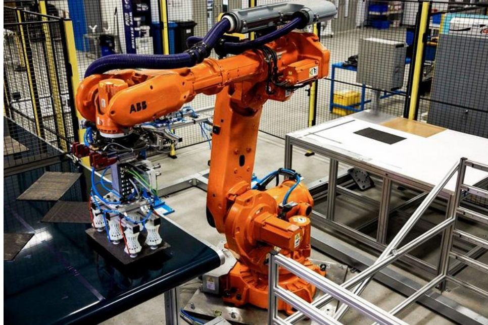
Figure 23: Example of a functional 3D printed gripper intricate design for a 5-axis pick-and-place robot 70
