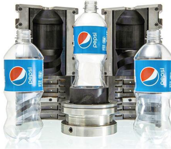
Figure 25: 3D printed injection mold insert to create a part prototype 74
